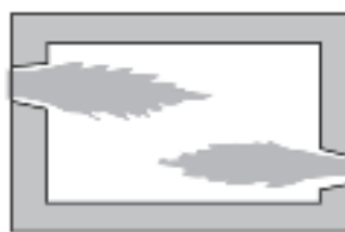
Figure 75: Correct heat distribution in furnace
