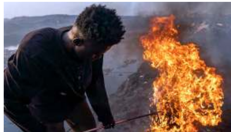
A young man in Ghana burns scrap electrical cables to recover copper after migrating from his village to Accra to engage in e-waste work.
