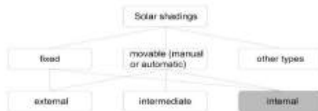
Fig. 1. Solar shading systems for buildings: a possible classification.
